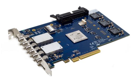
The Ndigo125M-14 is a high resolution x8 PCIe analog to digital converter operating at a sample rate of 125 Ms/s and a resolution of 14 bits. It supports onboard zero supression for pulse extraction on the input data stream. Two channels can be streamed at the full sample rate into the PC memory.
