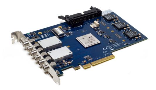
The Ndigo 250M-14 is a high resolution x8 PCIe analog to digital converter operating at a sample rate of 250 Ms/s and a resolution of 14 bits. It supports onboard zero supression for pulse extraction on the input data stream. Two channels can be streamed at the full sample rate into the PC memory.
