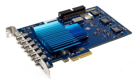
The Ndigo 5G-8 is a highspeed x4 PCle analog to digital converter operating at a maximum sample rate of 5 Gs/s and a resolution of 8 bits. It supports onboard zero supression for pulse extraction of the input data stream.
