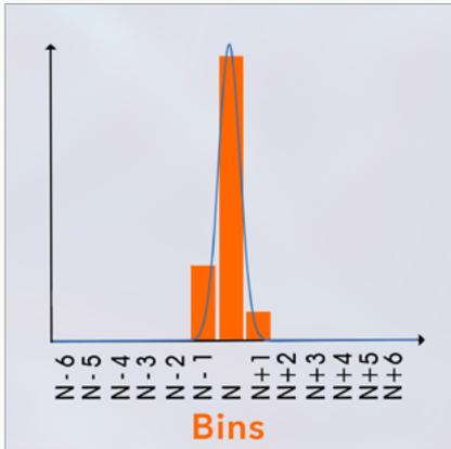
The occurring cycle to cycle jitter of the xHPTDC8-PCIe is much lower than the bin size of 13ps. Therefore you can expect an RMS error below 7ps for your measurements.
