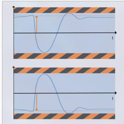
The threshold discriminators can use positive or negative threshold with configurable voltage. This allows you to use the xHPTDC8-PCIe with a wide range of detectors or constant fraction discriminators (CFD).
