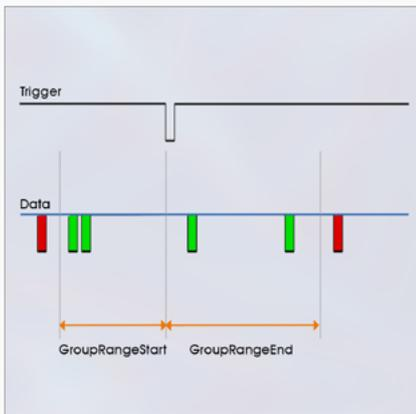
There is no limit in range of time measurement for this TDC. It will output an infinite stream of timestamps for all incoming pulses. In case you prefer common start or common stop the device can output structured data that mimic these modes.
